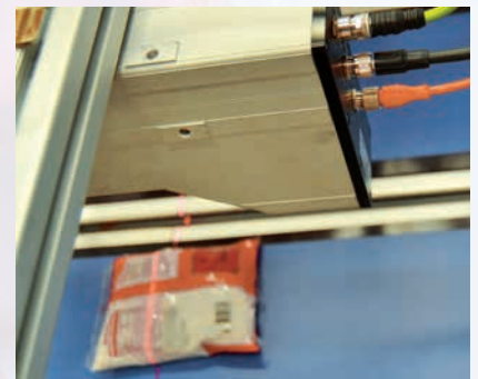
IVC-3D provides three-dimensional position data and timing information.
