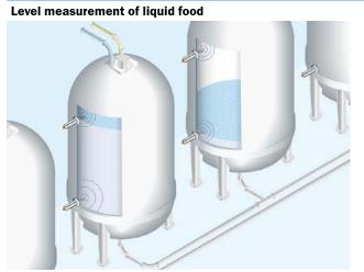
LFV200 is a universal sensor for the food and beverage industries that is used to monitor levels in storage and buffer tanks. It is also used for dry running pump protection. A compact design, high enclosure rate, CIP/SIP capability characterize LFV200 for hygienic applications.
