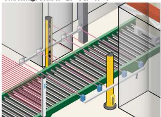
Point-of-operation guarding or access protection in industries that require cold storage, such as food and beverage and logistics, with temperatures down to -10 °C ... -40 °C.
