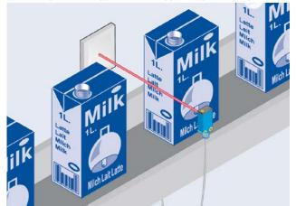
WL4-3: simple and quick alignment during commissioning. Reliable operation when contaminated due to high reserve factors. Also detects packaging with reflective surfaces.
