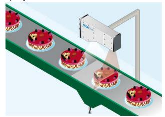
The IVC-3D smart camera records the 3D shape at high speed as the baked cakes pass by on the conveyor belt. The camera checks that the cakes have no dents or missing chunks, and that they have the correct height, volume, roundness and diameter. The version with a stainless steel housing makes it ideal for food and beverage applications.
