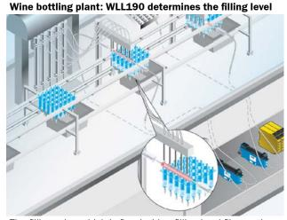
The filling tube, which is fitted with a filling level fiber-optic cable, is inserted down into the bottle neck, and filling begins. Once the desired level has been reached, the WLL190T-2 switches and the filling process stops immediately.
