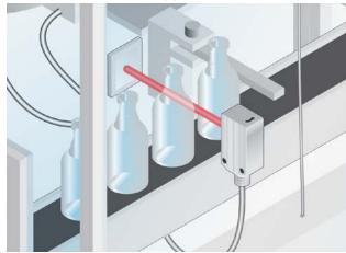
Recognition of PET and glass bottles under very harsh ambient conditions. The all around solution – reliable recognition of all packaging in the food and beverages market. Simple setting via Metal Membrane Teach. High reliability due to automatically tracking switching threshold.
