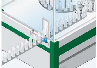
WL12G detects thin-walled, transparent bottles. It also recognises bottles which are lying down, i.e., are incorrectly positioned, and activates a pusher. This ensures that only bottles which are positioned correctly are fed into the bottler.
