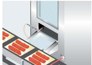
The IMF18 inductive sensor detects the presence of a tray at the tray magazine.
