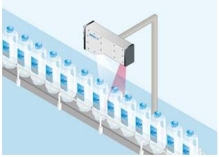
The IVC-3D smart camera locates the lid and verifies that it is correctly assembled. For many package types, the 3D measurements can be made relative to the rest of the package. This gives a correct result even if the container itself is slightly tilted on the conveyor.
