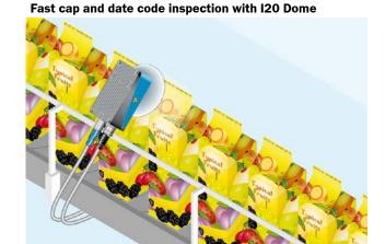
With the sophisticated Inspector part inspection tool set, verifying the presence of package details moving on a conveyor belt is as easy. Edge pixel counter inspection is used to check that the packaging has a code, while contour inspection is used to check that it has a cap.
