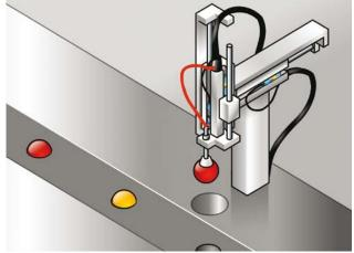
MZT8 detects the end position of the piston in a pneumatic cylinder/gripper, which serves as a pick and place application.
