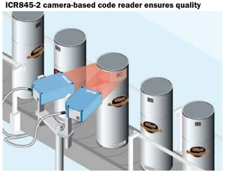
Data Matrix codes on the packages ensure goods are correctly sorted and guarantees high quality in the packaging process. TThe ICR845-2 code reader identifies all codes on the fly at a speed of up to 3 m/s and does not negatively affect the machine throughput.
