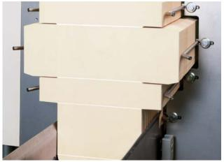
Task: to ensure that the aperture is sealed by the boxes. Solution: WTB4-3 sensor with self monitoring function. If the aperture is not sealed or if there is a sensor error, a message is sent to the control sytem.
