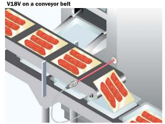
The VL18V photoelectric reflex sensor for transparent objects triggers the portioning belt for synchronizing the feed belt (packaging/transparent belts).
