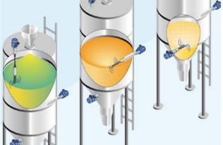
Level measurement and monitoring in raw material silos, such as overfill protection during filling or as a reliable minimum switch for emptying the silo. Robust and universal measuring technology for almost every raw material.
